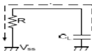
Fig. 3: Equivalent Circuit for Discharging Process in CMOS
